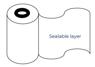
Food can be laid on the **AMISTYLE FT** film manually or automatically, taking care to match the product size with the film width. The product must not get inside the film sealing zone, as this may lead to loss of vacuum in the packaging
